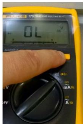
Fig. 5. Multimeter diode testing mode
